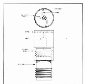
fig. 3. This coaxial diode multiplier mount is made from a female uhf barrel connector or an N barrel (UG-29B/U), a shell from a PL-259 connector, a piece of bare copper wire, and a 1N23 diode — simple and effective.
